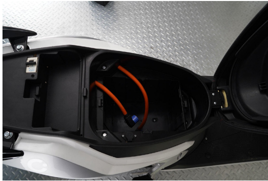
Fig. 18. Battery bottom connection
